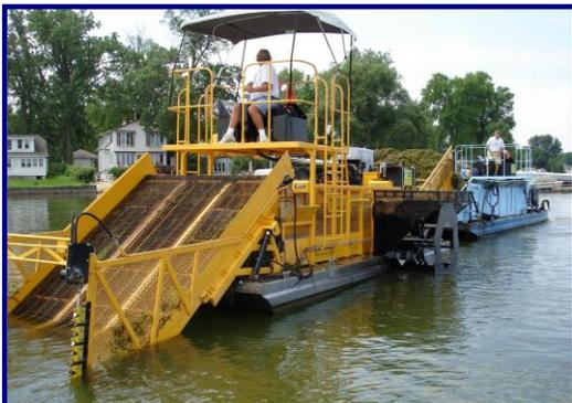
Whenever you are unloading into a transport barge, shore conveyor, or trailer conveyor, it is important to maintain the harvester's balance. To do so, lower the No. 1 input conveyor below the surface of the water. Once you are aligned with the transport, shore conveyor or trailer conveyor, raise the No. 3 discharge conveyor to hitch. Lowering the No. 1 input conveyor into the water serves as a keel and helps to stabilize the machine.
