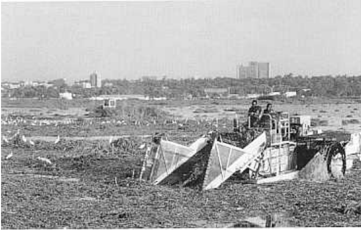
A medium-sized harvester cleans up the floating debris remaing from the chjopping work.
