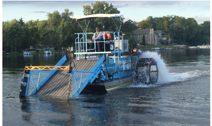
In Paddock Lake, a mechanical weed harvester removed 280 truckloads of aquatic vegetation from the lake - an estimated 2.2 million pounds of weeds.
